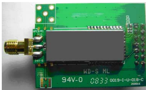
Figure 13. Top View of Dot-Power1000 Module with Shielding Case
