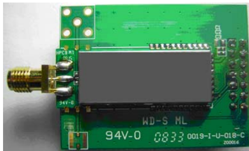
Figure 15. Top View of Dot-Power1000D Module with Shielding Case
