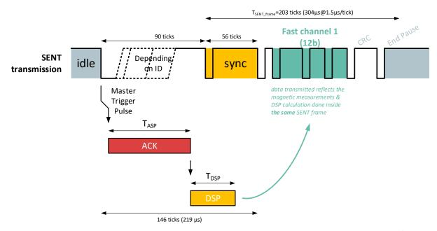
Figure 8 - SPC timing illustration in 1.5μs tick time mode and H.2 format
