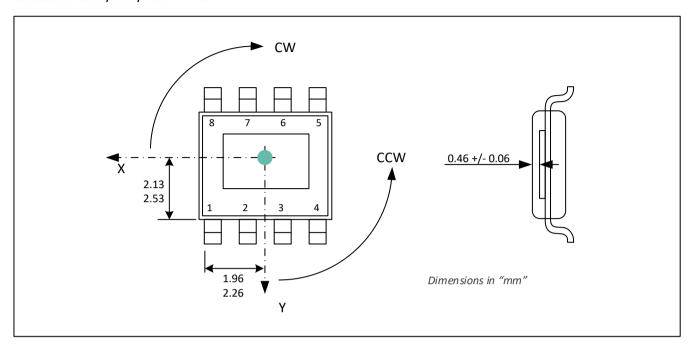
Figure 46 - SOIC-8 sensitive spot for rotary Stray-Field immune and standard/legacy modes
