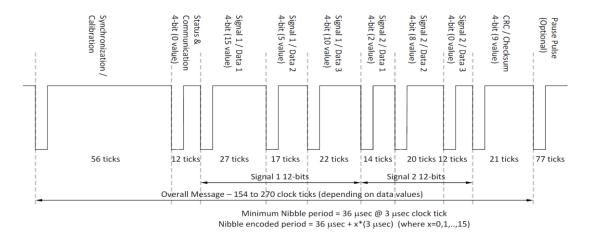
Figure 16 - SENT message encoding example for two 12bits signals
