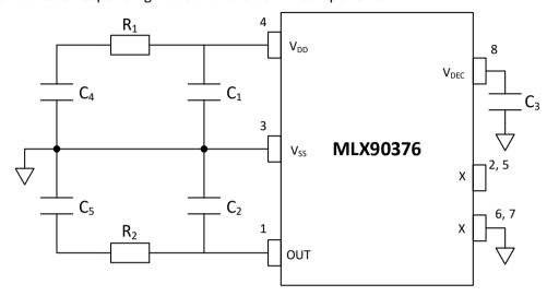
Figure 38 - Recommended wiring for the MLX90376 in SOIC-8 package
