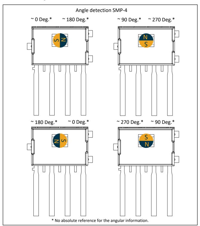
Figure 43 - SMP-4 Angle Detection
