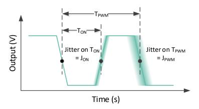
Figure 19 - PWM Signal definition
