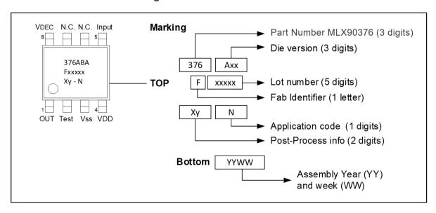
Figure 45 - SOIC-8 Pinout and Marking
