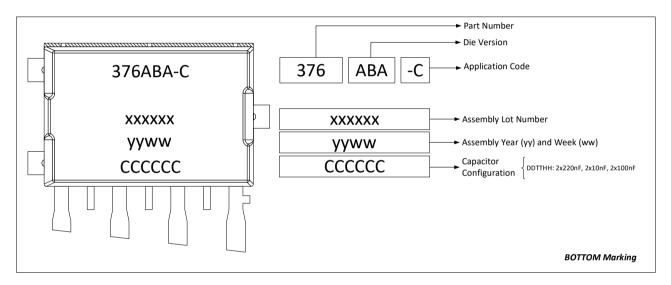
Figure 41 - SMP-4 Pinout and Marking
