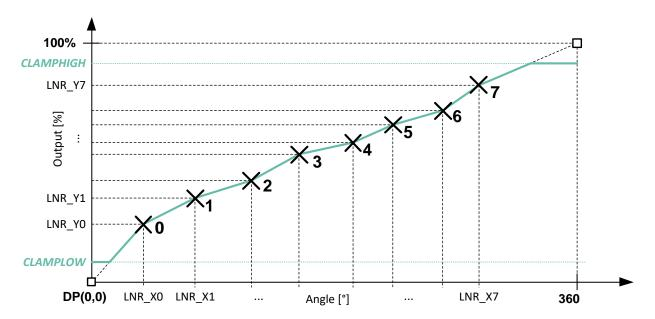
Figure 33 - 8-pts Linearization Parameters Description
