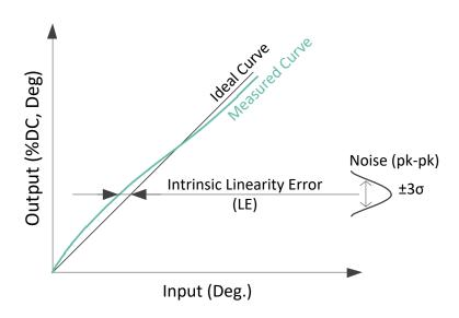
Figure 15 - Sensor accuracy definition
