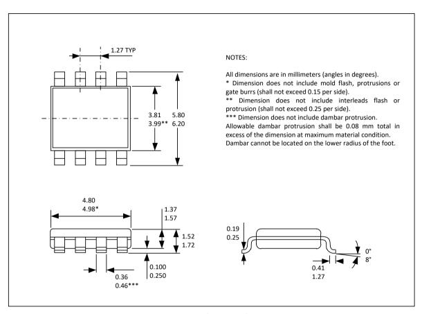
Figure 44 - SOIC-8 Package Outline Dimensions
