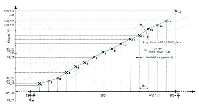
Figure 34 - 17-pts Linearization Parameters Description
