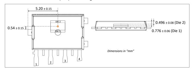
Figure 42 - SMP-4 sensitive spot for rotary Stray-Field immune and standard/legacy modes
