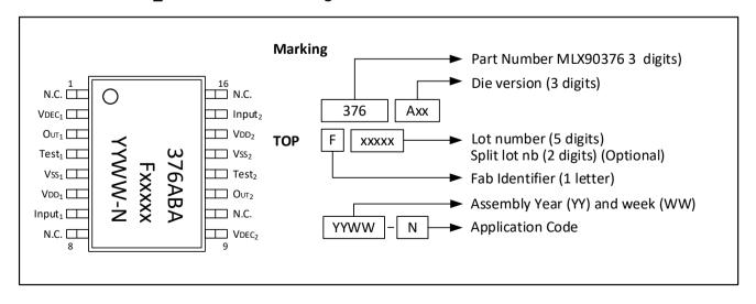
Figure 49 - TSSOP-16\_EP Pinout and Marking
