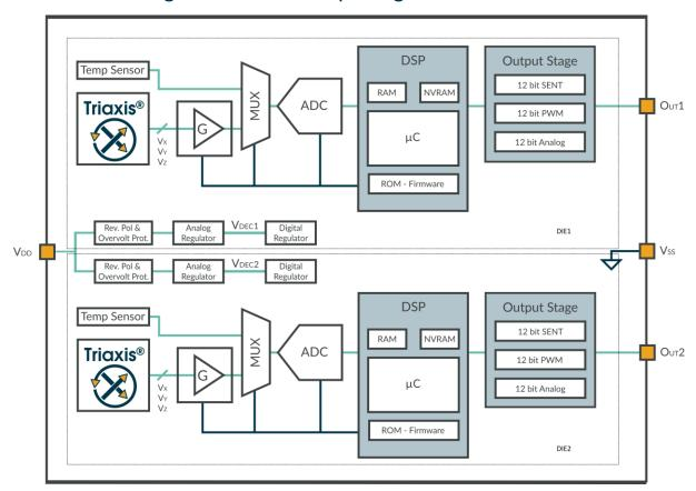
Figure 2 - MLX90376 Block diagram for SMP-4 package
