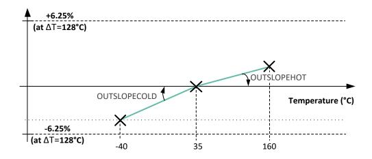
Figure 36 - Temperature compensated offset
