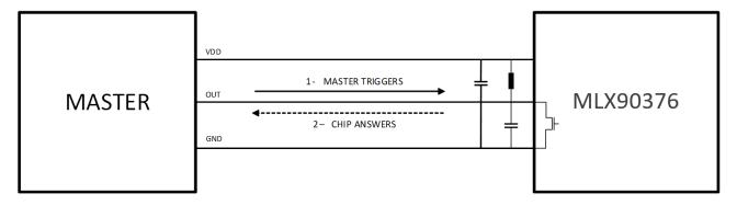
Figure 21 - SPC standard master-slave configuration
