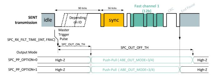
Figure 20 - SPC output driver state switching
