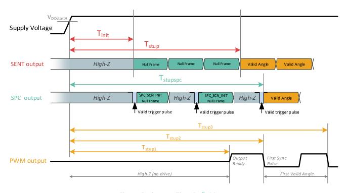
Figure 5 - Startup Time Definition
