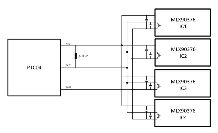
Figure 28 - Example of multiple units programming
