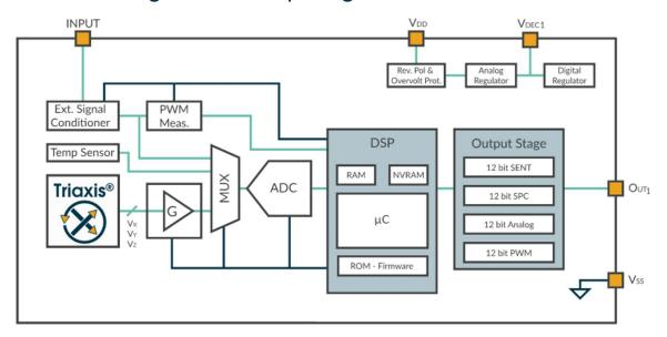
Figure 3 - MLX90376 Block diagram for SMD packages
