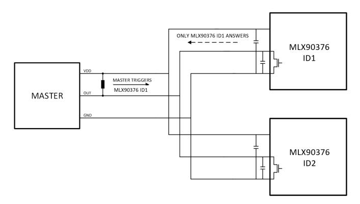
Figure 25 - SPC Bus Transmission Mode Multiplex Example
