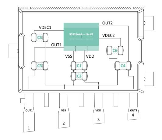
Figure 37 - Internal wiring of the MLX90376 in SMP-4 package
