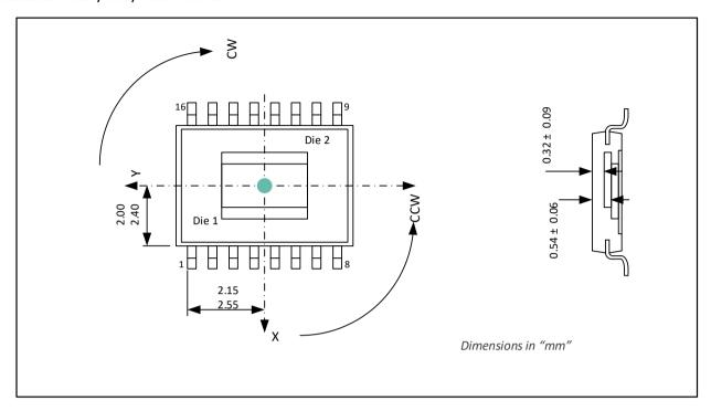
Figure 50 - TSSOP-16\_EP sensitive spot for rotary Stray-Field immune and standard/legacy modes
