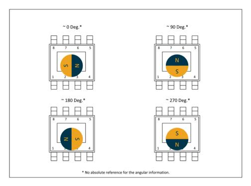
Figure 47 - SOIC-8 Angle Detection for MLX90376ABA
