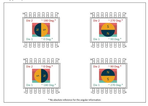
Figure 51 - TSSOP-16\_EP Angle Detection for MLX90376ABA
