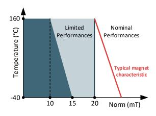
Figure 11 - Minimum useful signal definition for Standard/Legacy application
