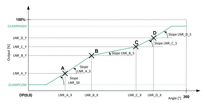
Figure 32 - 4-pts Linearization Parameters Description
