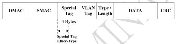
The detail information carried by received special tag is described as below. Through received special tag, CPU can tell switch the handle rule per frame over the internal setting. This feature can be enabled through REG 213H bit 6.
