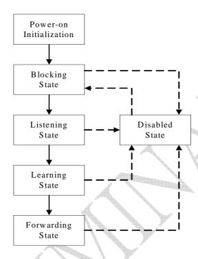
But in RSTP, there are only three port states. The port states comparison between STP and RSTP are listed as below.
