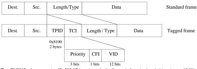
The DM9016 also supports 16 802.1Q-based VLAN groups, as specified in bit 1 of register 53h. It's obvious that the tagged packets can be assigned to several different VLANs which are determined according to the VID inside the VLAN Tag. Therefore, the operation is similar to port-based VLAN. The DM9016 used LSB 4-bytes VID of received packet with VLAN tag and VLAN Group Mapping Register (B0h~BFh) to configure the VLAN partition. If the
