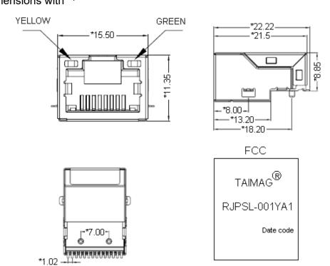
PCB LAYOUT: mm; TOLERANCE: ±0.10
