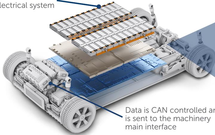
Data is CAN controlled and is sent to the machinery main interface
